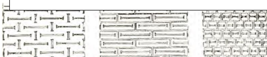
Fig 2: Brick construction methods on the walls inside and outside of the Samanid Mausoleum
